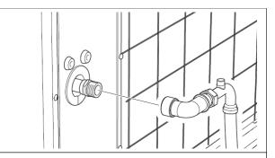
If the distance to the wall is short, mount an additional angle if necessary. The additional angle is to be provided, on site
