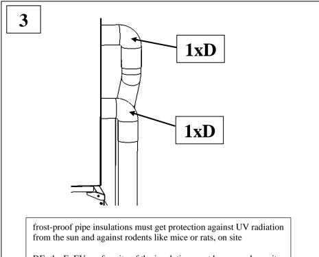
DE: the EnEV conformity of the insulation must be ensured, on site
