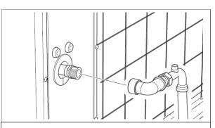
If the distance to the wall is short, mount an additional angle if necessary. The additional angle is to be provided, on site
